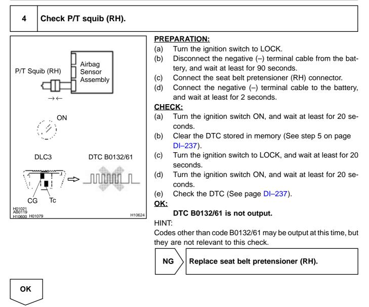
From results of above inspection, suspected part can now be considered normal. To make sure of this, use simulation method to check. If suspected part can not be detected by simulation method, replace all SRS components including wire harness.
